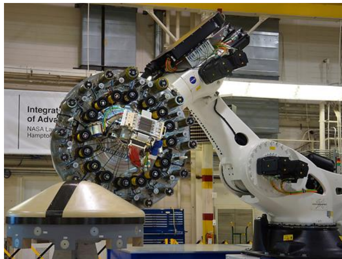
Figure 3. Electroimpact end effector on a robot arm
