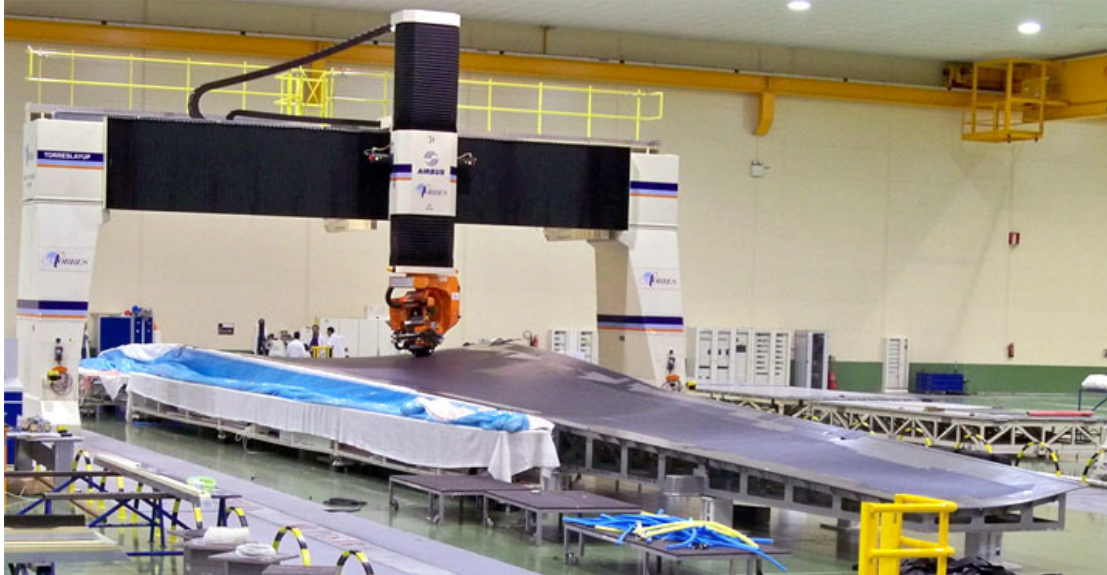
Figure 2. MTorres overhead gantry ATL machine
