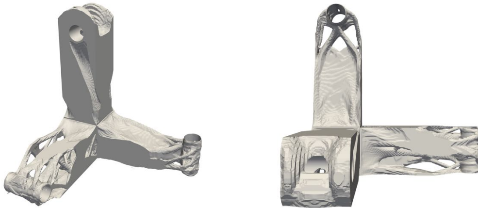
Figure 45: Isometric and top views of the stress-constrained mass minimization result for the orthogonal bracket problem
