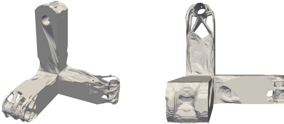
Figure 46: Isometric and top views of the stress- and frequency-constrained mass minimization result for the orthogonal bracket problem
