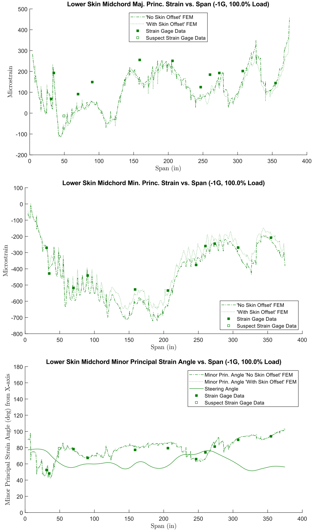
Figure C.29. Principal strains for lower skin mid-chord, -1G: major, minor and minor angle.
