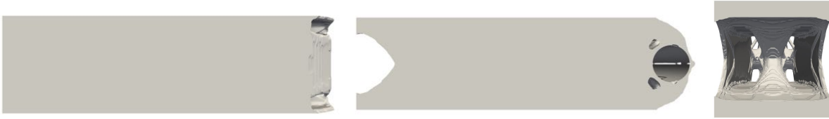
Figure 36: Top, side, and rear views of the mass-constrained compliance minimization result for the cantilever beam problem
