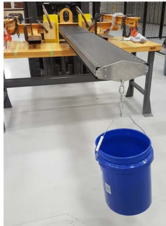
Figure 7. Cantilevered Load Test. Supported by forklift resting on table. Deflection measured with laser tracker at 8 points (4 span locations x 2 chord locations).
