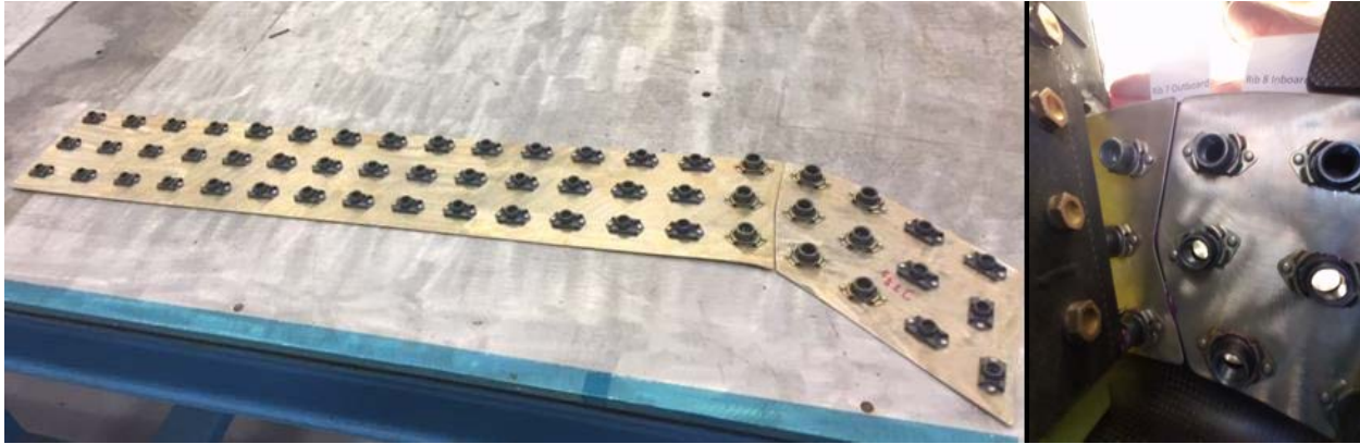
Figure 5.7. Nutplate carrier assembled (left) and installed (right).
