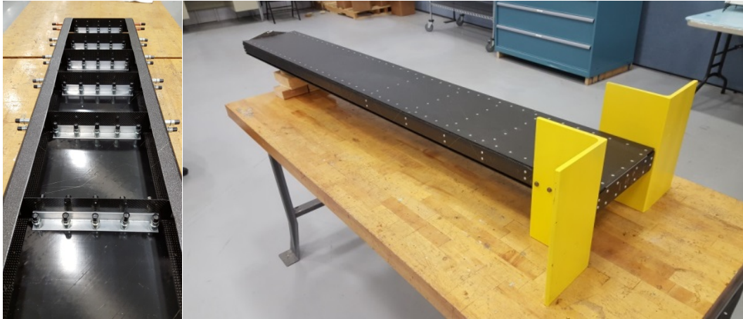
Figure 2.5. Partial assembly of Hershey wing box (left) and final assembly (right).
