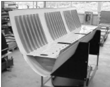
The A380 wing fixed leading edge will be produced from fiberglass/PPS thermoplastic prepreg supplied by Ten Cate. The technology was first proven on the A340-600 leading edge, shown here.
