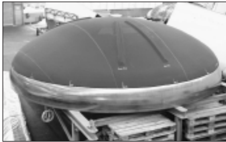
A full-scale (5.5m by 6.2m/18-ft by 20.3-ft) A380 rear pressure bulkhead, produced from CYCOM 977-2 epoxy and Saertex non-crimp carbon fiber fabrics using the resin film infusion process.
