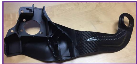
**Figure 2: Finished Composite Knuckle-Tie Blade**
