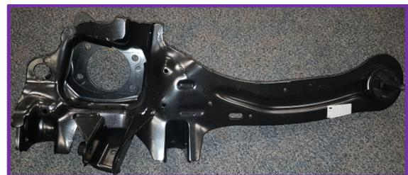
**Figure 1: Steel Knuckle-Tie Blade**
