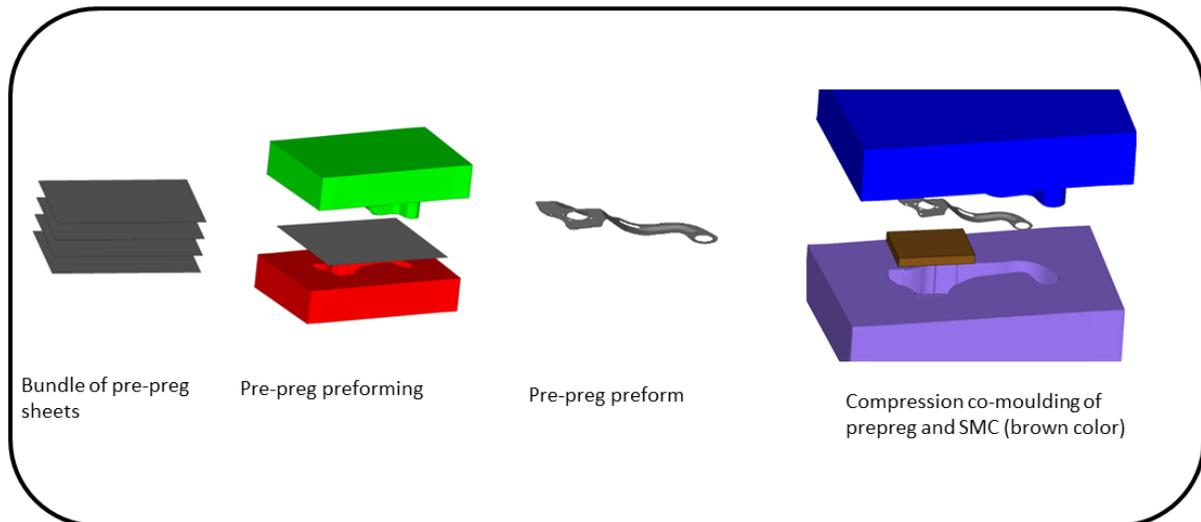
**Figure 3: Steps in the manufacture of composite part**
