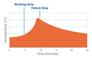
Figure 3: This graph of exotherm temperature vs time at room temperature shows the fast cure of an MMA adhesive.
