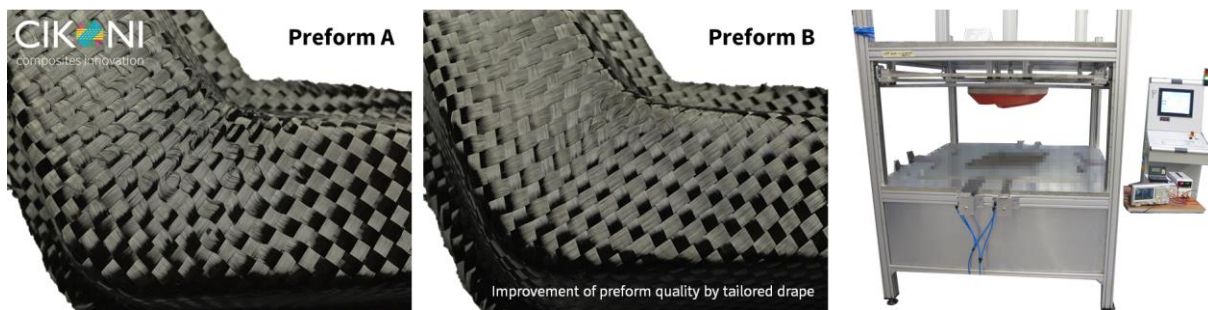
Figure 3: Preform variations using the example of an L-shape and preforming device with single-layer material guidance for small volume production
