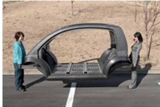
Carbon fiber has 10 times the strength but just a fourth of the weight of steel. Composite materials made of carbon fibers and resins are already widely used to reduce the weight of aircraft and other industrial materials. However, conventional thermoset-formed carbon fiber composites are rarely seen in mass production due to its slow takt time.
