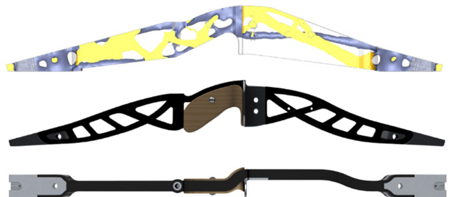
Top: Result of the topology optimization Middle and bottom: Side and top view (CAD model) of the new developed riser
