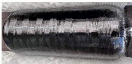
Figure 8: Completely wound and cured vessel
