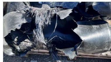
Figure 9: Vessel after burst testing
