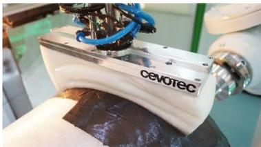
Figure 6: Placement of local dome reinforcement patches with FFP
