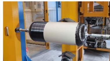
Figure 7: Winding of dome reinforced Type 4 tank
